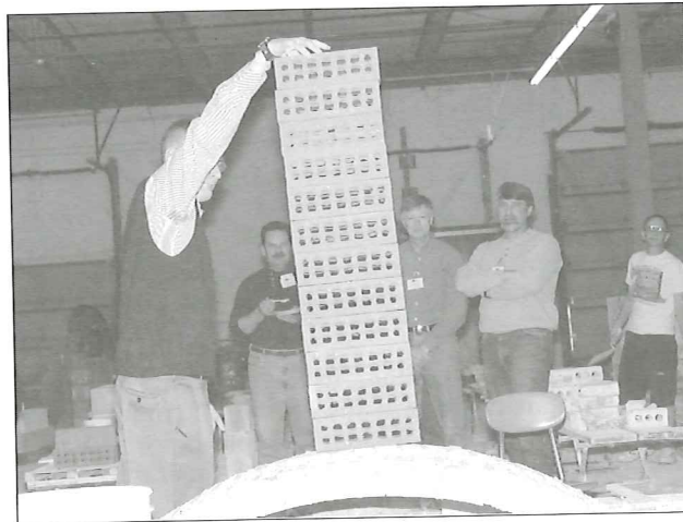
How much weight can be borne by an arch? IMI Wisconsin Area Director of Market Development Pat Conway adds to a stack of bricks as workshop participants watch for collapse. The arch, on which the mortar was still green, supported 14 bricks, or about 160 pounds, before it gave way.
